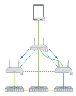
Figure 2: Distributed Controller Architecture
